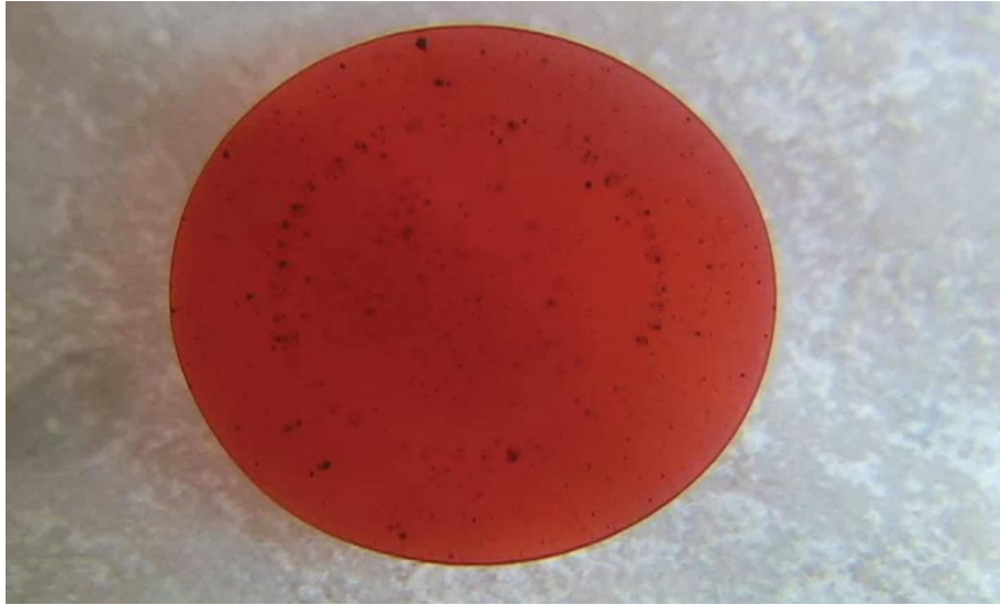
Figure 18.5: An oil drop oscillates on the water surface. Note the ring of impurities that marks the edge of the internal circulation.
