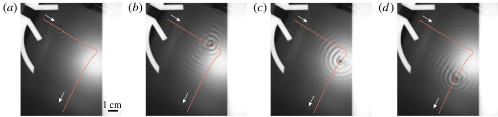
FIGURE 2. Four snapshots of a walking droplet with its wave field as it is reflected from a submerged barrier (in white). (a)  $t = 1.2$  s, (b)  $t = 4.4$  s, (c)  $t = 7.1$  s, (d)  $t = 9.4$  s.
