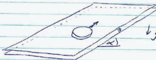
$$\frac{\text{DISSIPATION}}{\text{AREA}} = \frac{\Phi_{\text{loss}}}{A} = 2\mu \int_{-h}^h \left( \frac{\partial u}{\partial z} \right)^2 dz$$
