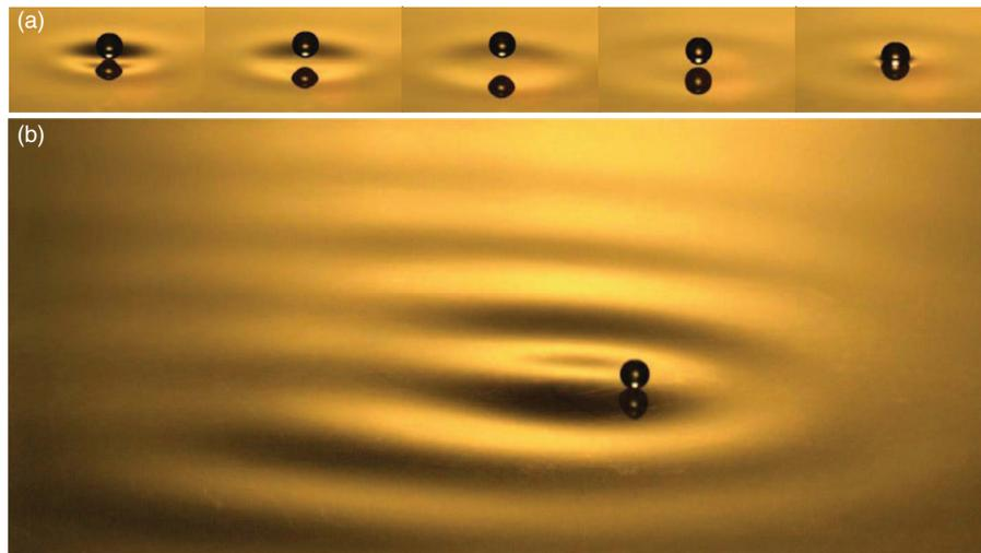
FIG. 1. (a) An oil droplet bouncing in place on a vibrating fluid bath. (b) At higher forcing amplitude, the droplet walks across the surface of the bath, propelled by its pilot-wave field (enhanced online). [URL: <http://dx.doi.org/10.1063/1.4820128.1>]
