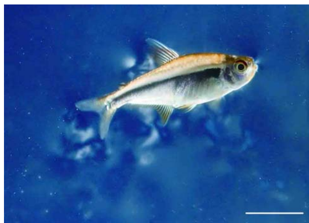
Fig. 3 A black neon tetra fish flaps its fins in a TMV solution. The luminous areas are indicative of the fluid shear generated by its fins and inhalation by its mouth. Scale bar 1 cm
