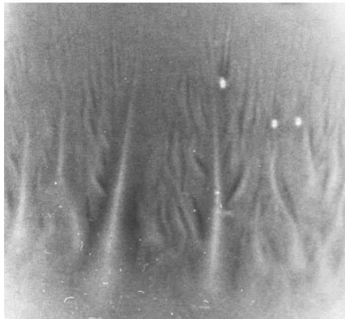
FIGURE 6. Plan view of the dendritic free-surface structure evident in a 50% methanol, 50% water solution climbing a 3° slope. The flow is from bottom to top, and the horizontal extent of the image is 5 cm. The free surface deformations are rendered visible with a shadowgraph.
