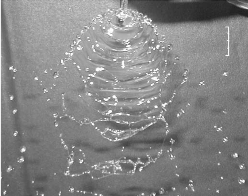
FIGURE 13. A typical snapshot of the flow taken in the ‘violent flapping’ regime delineated in figure 11. The sheet disintegrates into a series of droplets due to the large-amplitude flapping instability of the sheet. Scale bar: 1 cm.
