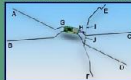
[Conceptual 3-D CAD model of the water strider robot. A, B, C and D are the supporting legs; E and F are the actuating legs; G is the body with sensors, power sources and a wireless communication module; H is the middle actuator; and I and J are the right/left actuators.]
