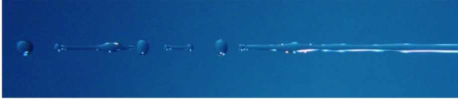
Figure 3: Breakup of a fluid thread
