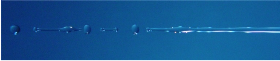
Figure 3: Breakup of a fluid thread
