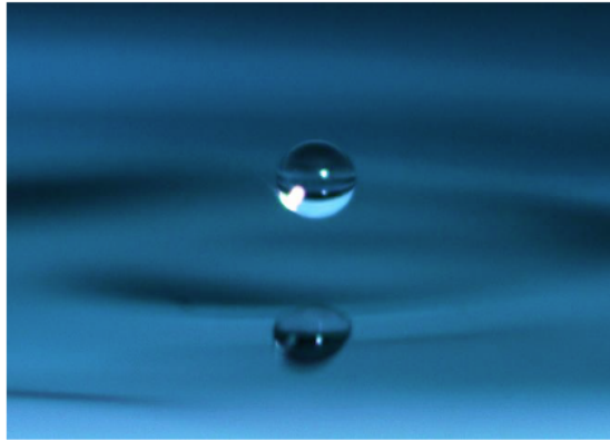
Figure 5: Droplet bouncing on a vibrating bath of silicon oil.
