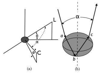
Fig. 1. Geometry used to photograph falling drops. (a) Ellipsoidal drop at the origin with its symmetry axis vertical. The light source is located at *L* at an angle  $\theta$  above the horizontal. The camera at *C* is at an angle  $\phi$  above the horizontal plane. The scattering angle  $\alpha$  is the angle between the light source and the observer at *C*. (b) Rays propagating inside the drop.
