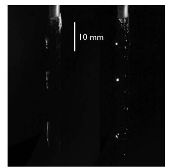
Fig. 3. Time exposure of a water drop on the left, and a stroboscopic image of a drop under the same conditions of flow rate on the right.
